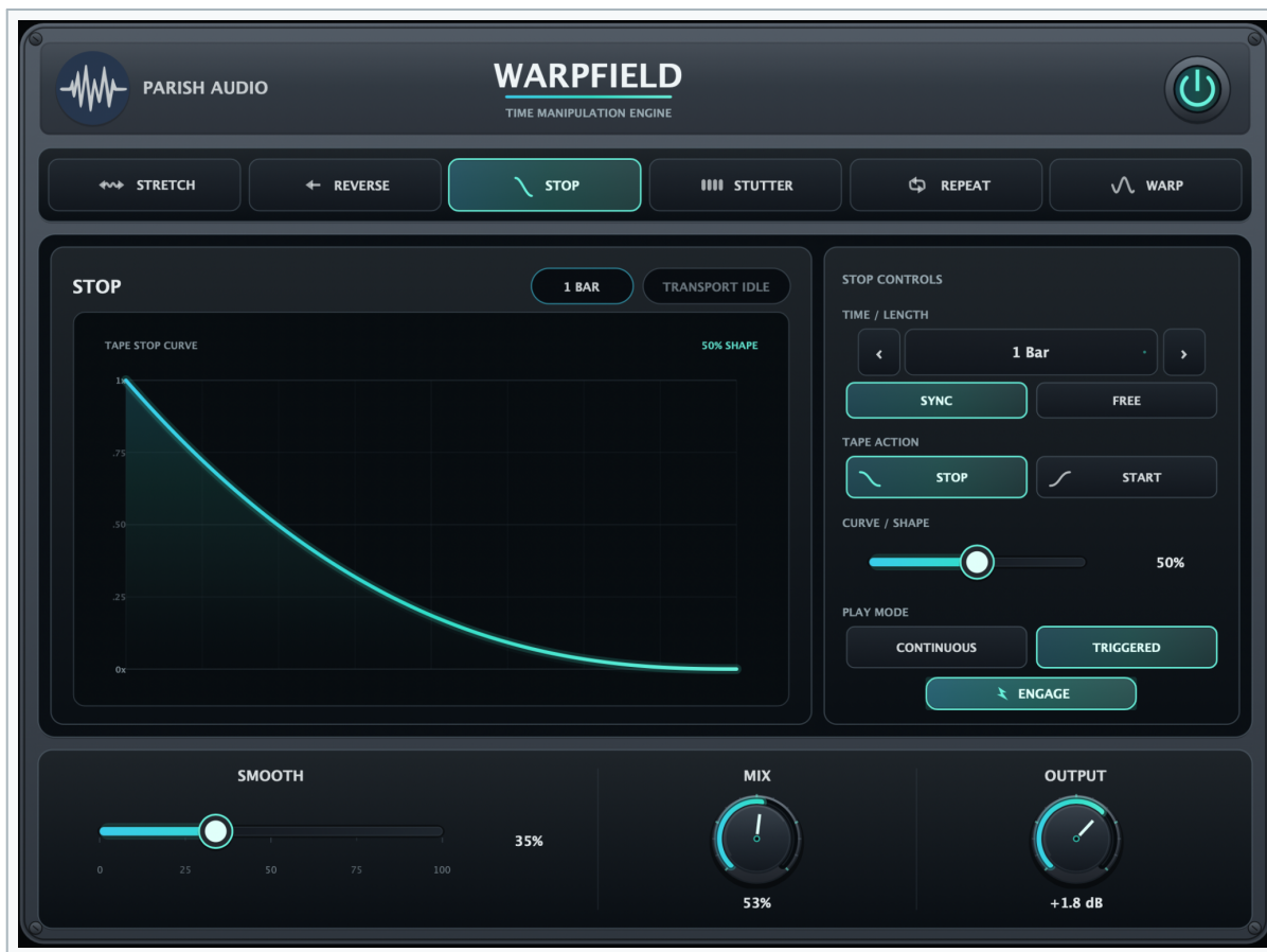
Stop mode - the display shows the tape-speed trajectory used by Tape Stop or Tape Start.
