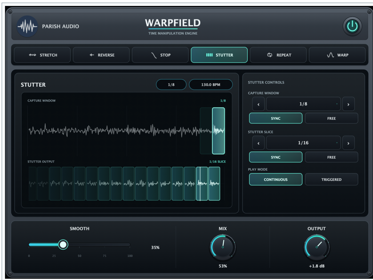
Stutter mode - a recent tail slice is repeated inside the larger capture window.
